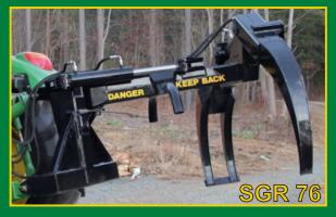
VALBY® SGR 76 Tractor Grapples are built using a bypass design whereby the single tine on one side of the grapple passes through the gap between the double tines on the opposite side of the grapple. The tines tighten up completely on the load, keeping it balanced and in control. The result is that logs are easily picked up and "rolled in." The SGR 48 is designed for lighter duty work, and accomplishes the same task using one tine on each side.
